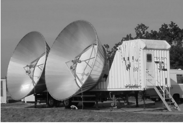
Fig. 1. The TARA system. Clearly visible are the multiple feed systems to generate off-axis beams.
