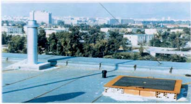
Fig. 1. The installation of the Disdrometer RD-69 on the roof of the Water Resources building.
