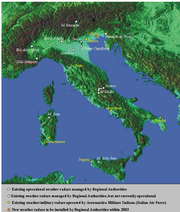
Fig. 1. Status of the Italian radar coverage as classified at 31 December 2001 – The colored-symbol legend explains the owner institution (i.e., Regional Authority, Air Force, Research Institution) and the current status of each radar system (i.e., operational, not operational, to be installed).
