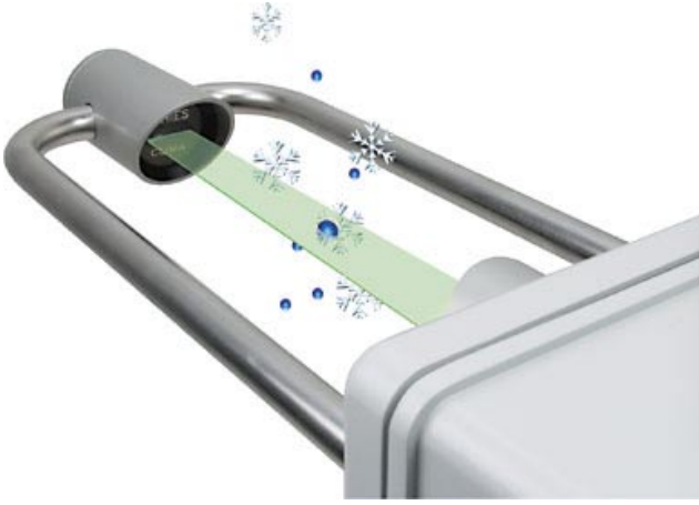
Fig. 1. Explanation of the measuring principle of LPM.
